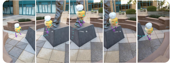
Figure 7. With localized depth, DepthLab can automatically plan a 3D path for the avatar that avoids a collision with the statue by making the avatar hover over the statue.
