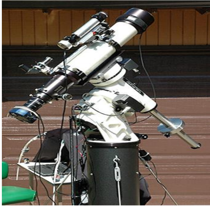
Fig. 1. Telescopes do not just look at a star. Most of the time, a spectrometer is attached to the telescope. This telescope is fitted with a diffraction grating of 500 lines/mm which is used to disperse the star-light into a spectrum.
