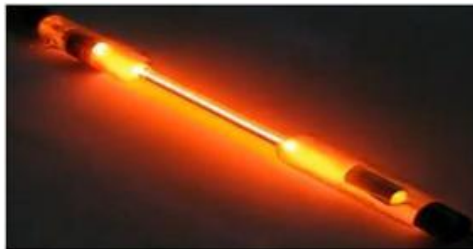
Fig. 13. The glow produced from neon atoms in when a high voltage is applied to a spectral tube containing neon atoms.
