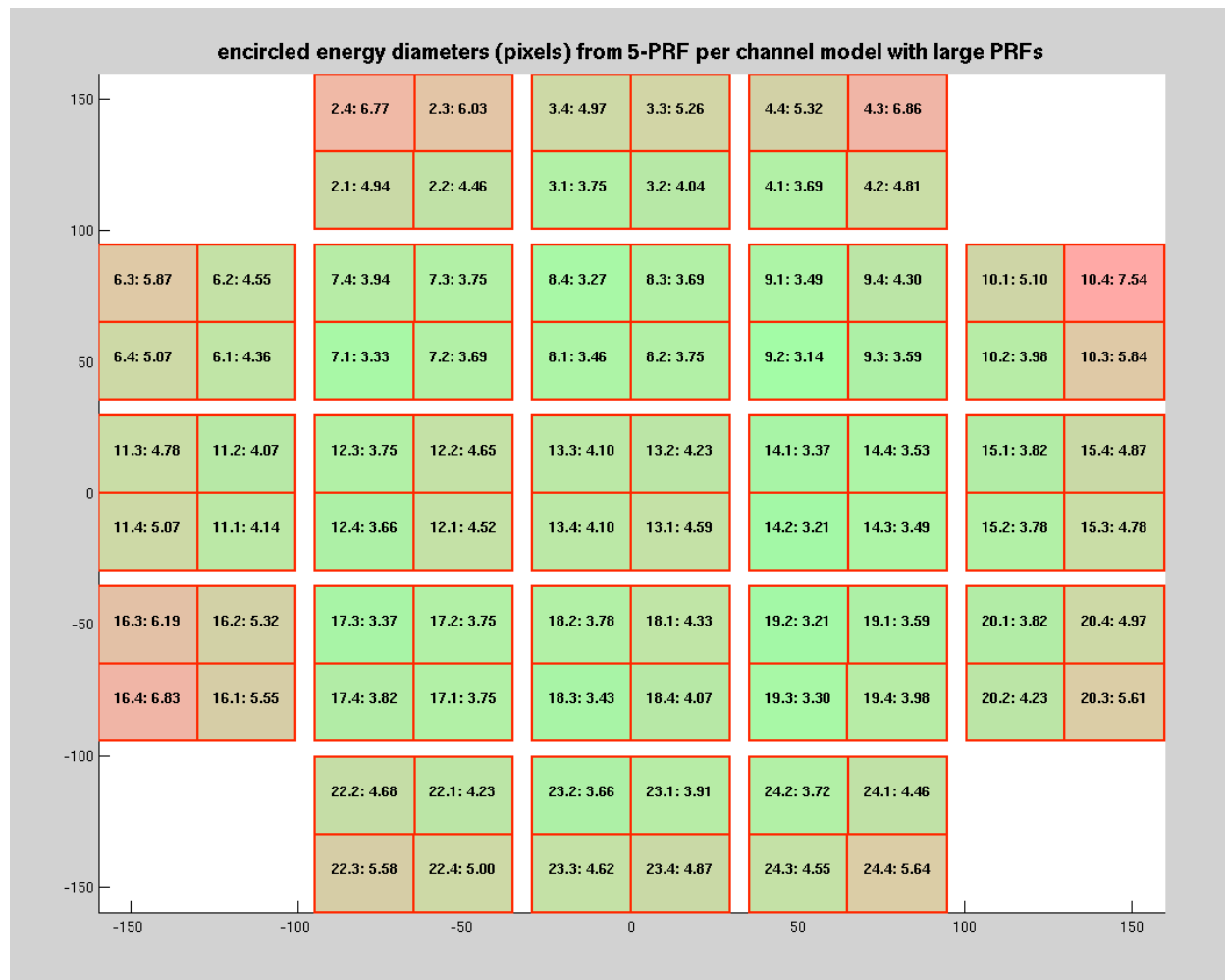
Figure 17: Observed 95% EE diameter after focusing the Kepler telescope (from Bryson 2009), arranged in the FPA co-ordinate system. Each box is labeled with the mod.out, followed by the 95% EE diameter in pixels. Green indicates a 95% EE diameter well within the 7.0 pixel requirement, shading to red in those few cases where the requirement is approached or slightly exceeded. The white corners indicate FGS channels.
