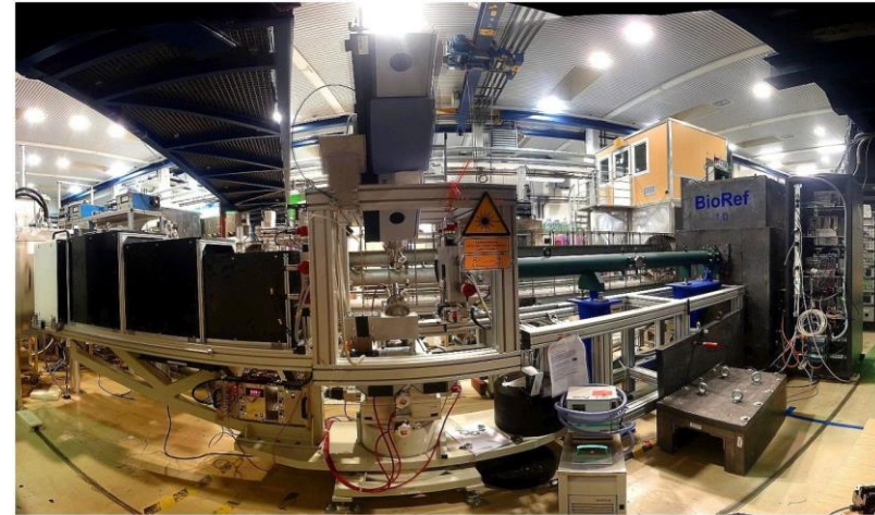
A fish-eye perspective of the new BioRef neutron reflectometer at the neutron source BERII at the Helmholtz Zentrum Berlin with the sample position in the center. The neutrons are guided through a chopper system from the right side and are detected with a position sensitive detector on the left side. As a special feature an infrared beam line is installed on the sample stage, with an infrared spectrometer on top, in order to perform combined infrared spectroscopy and neutron reflectivity measurements. The software
